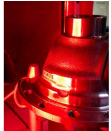
XL-Box laser machine with integrated vision in the marking head
